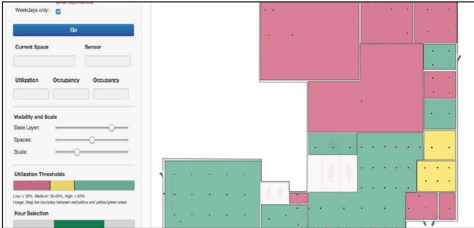
Luminaries commissioning – floor map view
